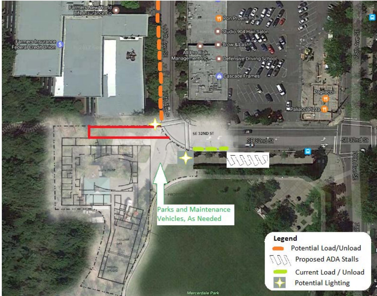
Figure 2 Load / Unload, ADA and Park Maintenance Areas
